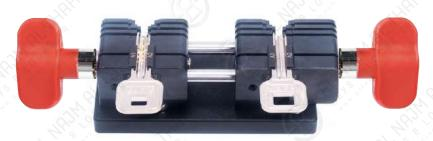
Clamp Jindian Yuanzi dimple key with A1+A2 lock blocks pushing to the bottom, no need stopper, to position key's shoulder, and press flat the key to clamp
