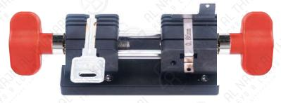
Put a 0.86mm shim on the fixture first, then clamp Jindian Yuanzi external milling blade key on the shim, and the stopper is placed in the first slot to position key's tip
