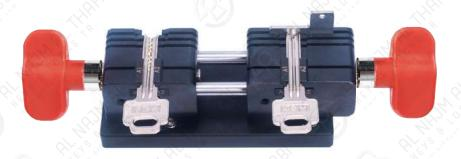
Clamp Baodean semi-circle dimple key with A1+A2 lock blocks pushing to the bottom, the stopper is placed in the first slot to position key's tip, press flat the key to clamp
