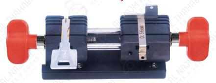
Put a 0.56mm shim on the fixture first, then clamp Jusen external milling double blade key on the shim, and the stopper is placed in the first slot to position key's tip
