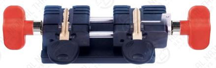
Clamp Hyundai Elantra external milling key with B1+B2 bilateral clamping, and the stopper is placed in the fourth slot to position key's shoulder
