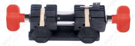
Clamp BMW key with A2 lock block to clamp one side, and the stopper is placed in the second slot to position key's tip.
