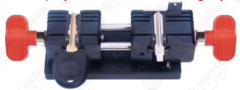
Clamp Hyundai Kia external milling keys with B1+B2 lock block bilateral clamping
