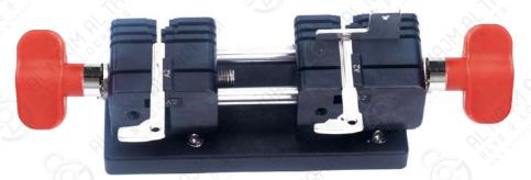
Clamp Mercedes-Benz key with A2 lock block to clamp one side, and the stopper is placed in the third slot to position key's tip.
