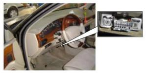
\*GM Buick: the OBDII plug is below the dashboard, use OBDII-16 connector.
