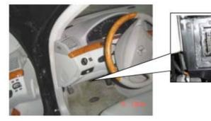
\*Benz S320,220 Chassis: the OBDII plug is below the dashboard, use OBDII-16 connector.
