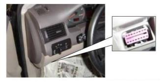
\*AUDI A6: the OBDII plug is on the lower left side of the dashboard, use OBDII-16 connector.
